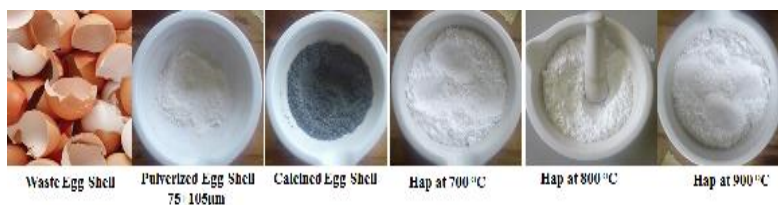
Fig. 7: Images of the pure HAp produced from waste poultry egg-shells for biomedical applications ( Baba et al., 2020c )
