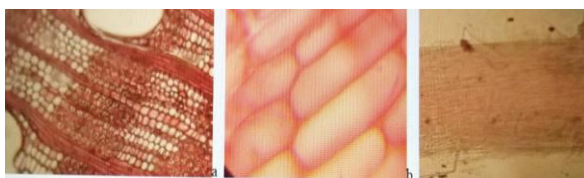
Fig. 7: Transverse section (a), transverse longitudinal section (b), and isolated fibres (c) of Ficus exasperata wood
