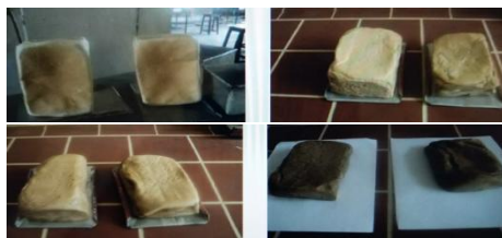
Fig. 6: Fibre-rich bread containing varying amounts of wood fibres (a – 0 g, b – 0.25 g, c - 0.5 g, and d – 1 g)
