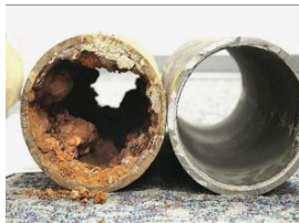
Figure 4B: Water pipe with narrowed bore (image on the left) which will reduce water flow (analogous to ischaemic stroke) ( https://www.therecord.com/news/waterloo-region/2015/01/21/aging-water-system-in-kitchener-means-big-rate-hikes-or-more-water-main-breaks.html Accessed 27 February, 2023).
