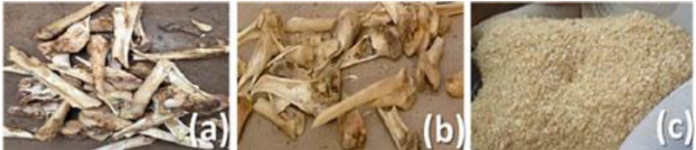
Figure 7: Bovine bone samples: (a) as sourced; (b) washed and cleaned; and (c) pulverized.
