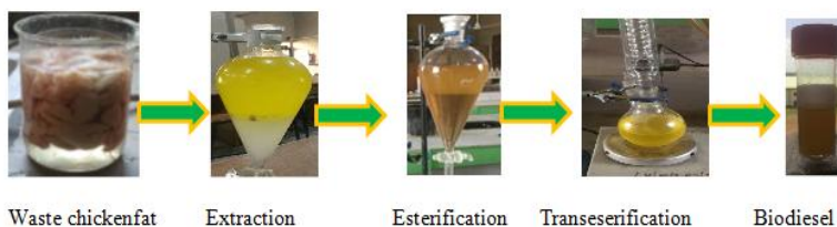
Figure 11: Biofuel production from waste chicken fat and egg shell (Odetoye et al. , 2021)
