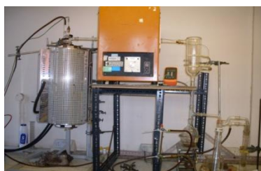
Figure 8: Experimental set up for intermediate pyrolysis experiment (Odetoeye et al. , 2018)
