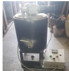
Figure 15: Wireframe AutoCAD design view and fabricated melt-mixer (Odiase and Odetoye , 2022)
