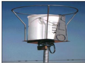
Figure 7: Single open bucket sampler (ASTM D1739, 2010; Nwosu, Abdul Raheem and Shehu, 2016)
